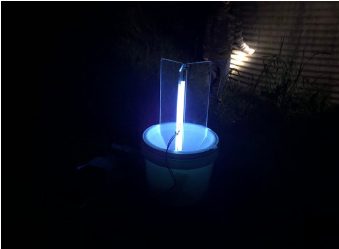
Figure 3: Robinson Trap in use, showing illuminated black light bulb and perspex panels
